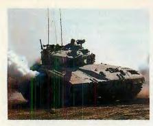
ABOVE: The Merkava's business end; currently fitted with a 105mm cannon, the Merkava will also accept 120mm and 130mm guns. RIGHT: Secondary armament on the Merkava includes twin roof-mounted FN MAG 7.62mm machine guns, a 7.62mm coaxial machine gun and a 60mm roof-mounted mortar.
